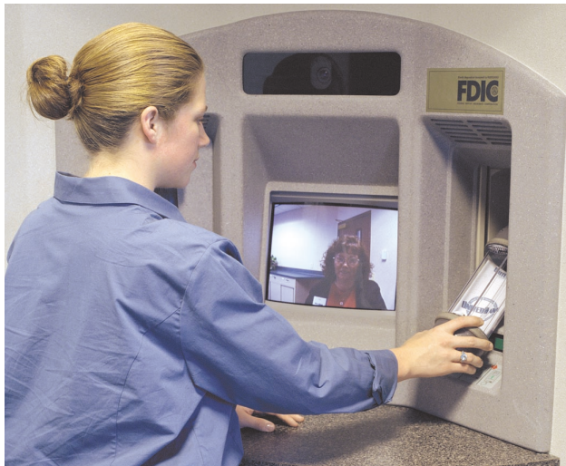
With a remote teller system, tellers work in a separate location and interact with members via video, telephone, and pneumatic tubes.
